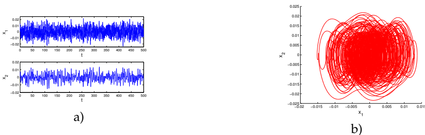
FIGURE 4. The time series of the coordinates and trajectory of the solution x(t) of equation (4.28), with Markovian components obtained for h = 0.1\pi . The stochastic influence is strong, since of the time step of the Markov chain is smaller than the period.
